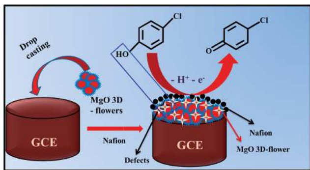
Scheme 2 Schematic representation of the surface modification of the GCE and proposed working mechanism for the detection of 4-CP.
