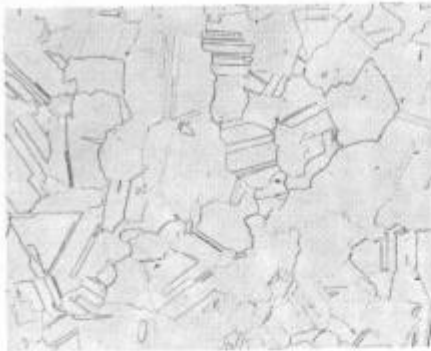
Figure 1. Microstructure of Hastelloy Alloy C-276 in as-received condition.
