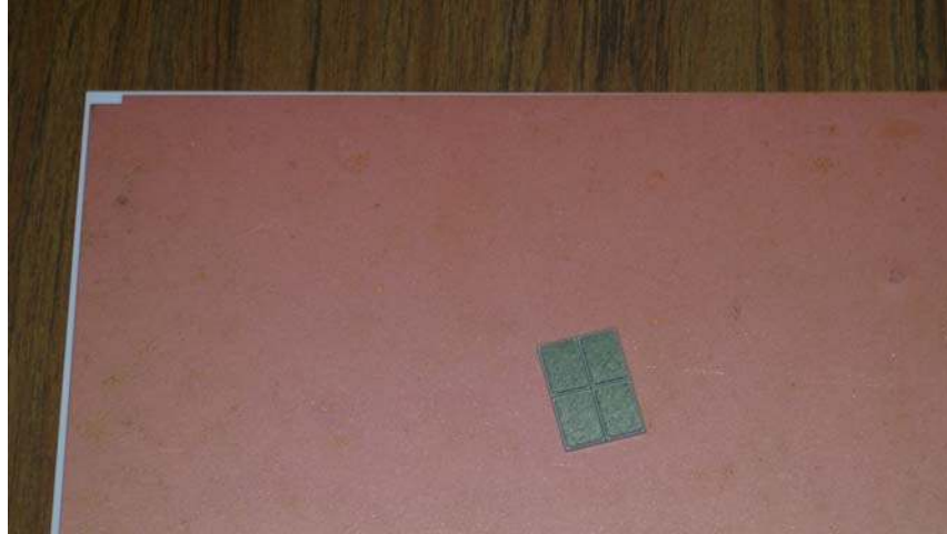
Fig. 1. A pane of DBC on Alumina and a small etched Ni plated DBC on AlN board.
