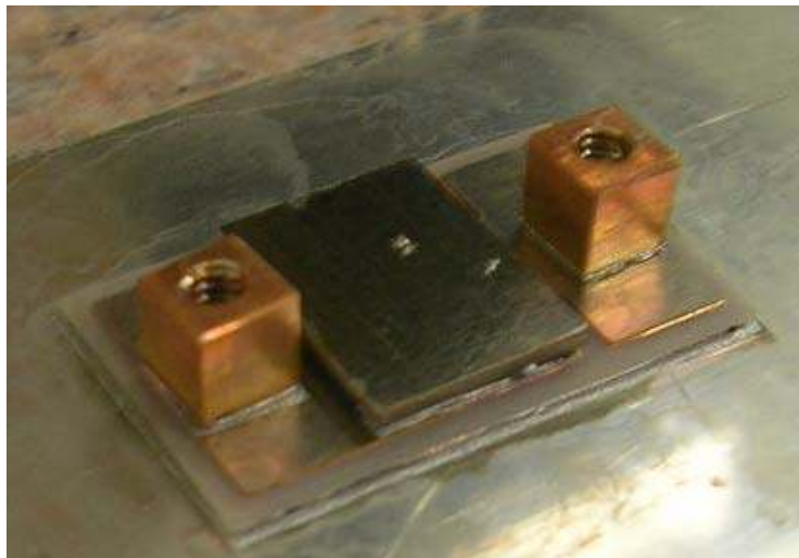
Fig. 9. A prototype flip-chip package.
