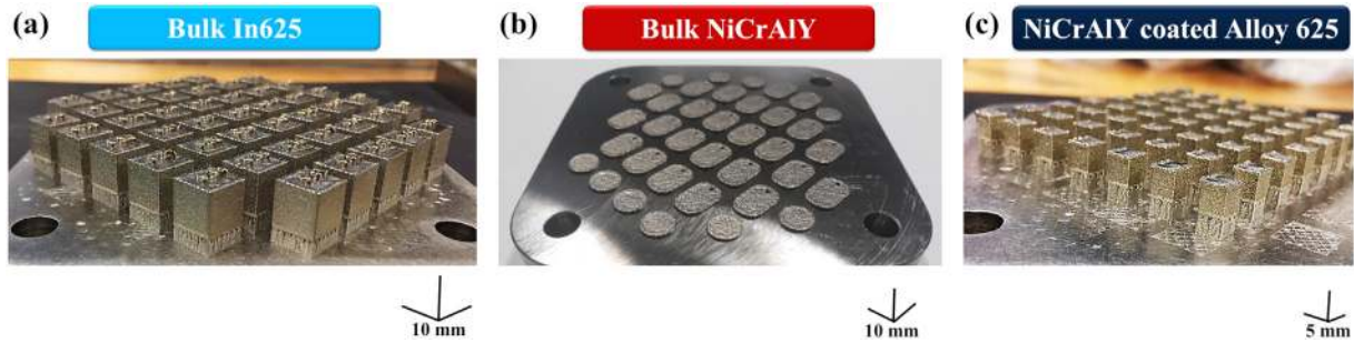
Fig. 1. Sample geometry for the three materials: (a) bulk Alloy 625, (b) bulk NiCrAlY, and (c) NiCrAlY coated Alloy 625 samples.
