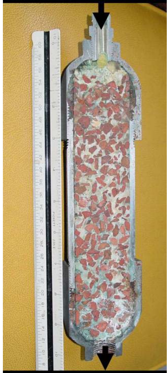
Figure 5. A gravel-packed pipe sample (post test). Arrows indicate water flow and grout injection direction.
