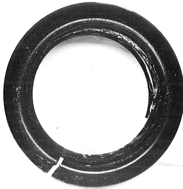
Figure 4. - Inboard element from one-inch polyimide 45° V-seal after 1358 hr duty cycle test at 500° F showing circumferential and radial cracks.
