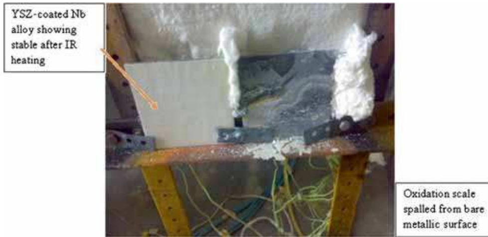
Figure 6. YSZ coated (600 \mu\text{m} ) (left) and uncoated (right) specimens after exposure to 1250°C for 30 s in atmospheric conditions.
