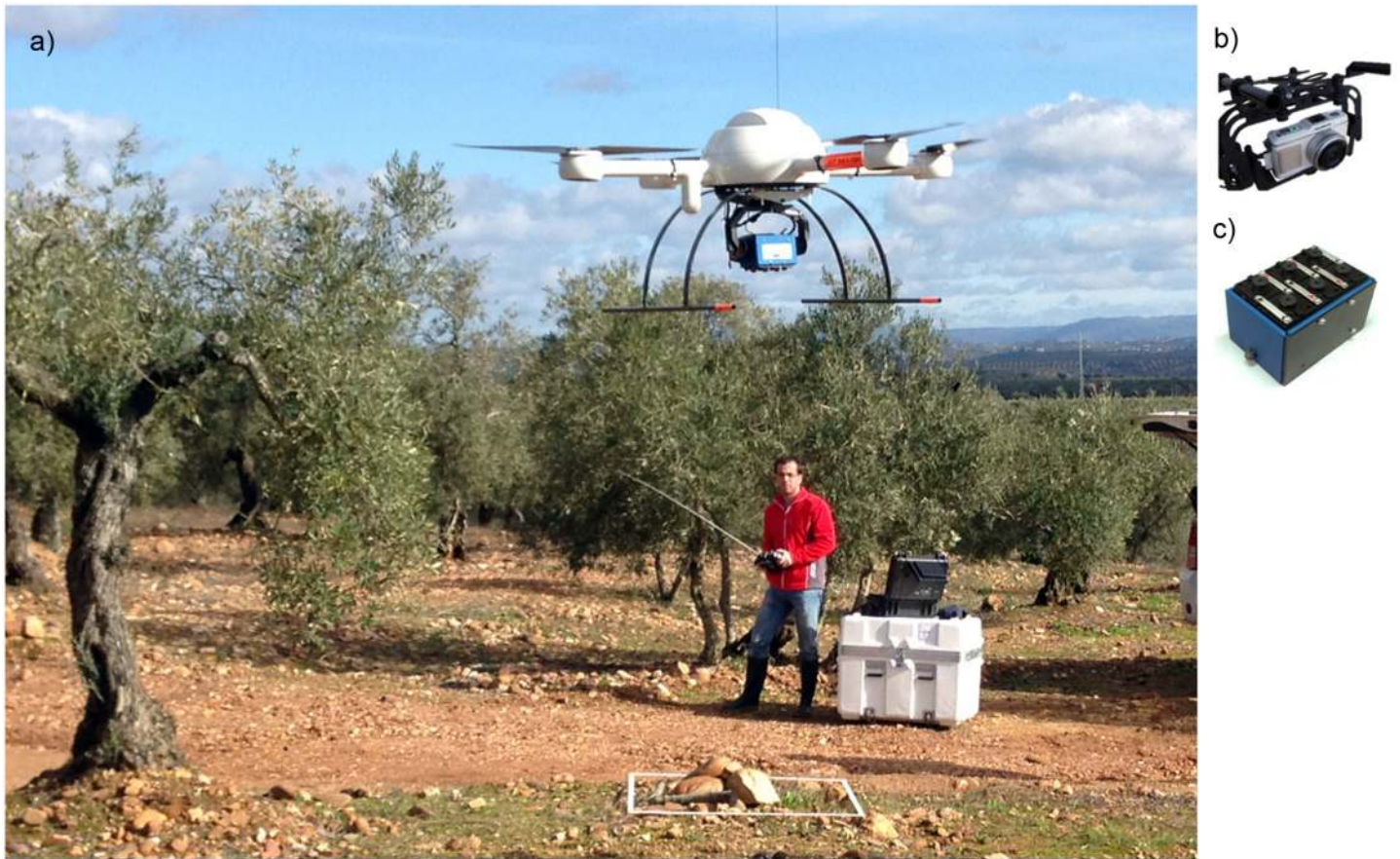
Fig 2. The quadcopter UAV, model md4-1000, taking off in one of the studied fields (a) and the sensors used in this investigation: the visible-light camera (b) and the multispectral camera (c). The individual in this figure has given written informed consent to publish his photograph.
