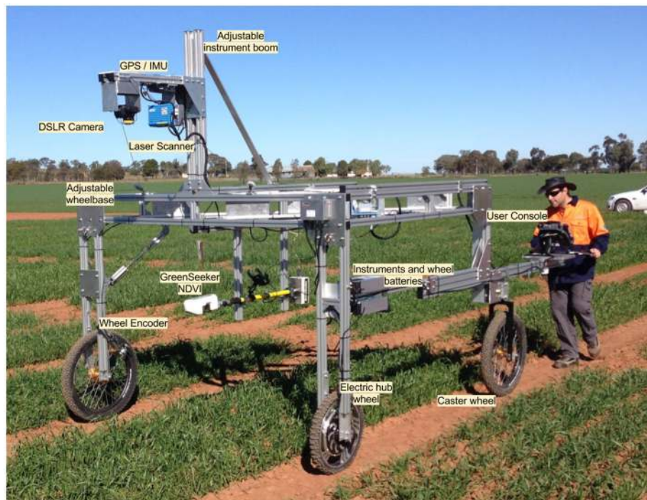
FIGURE 1 | Phenobile Lite comprising LiDAR laser scanner, digital single-lens reflex (DSLR) camera, GreenSeeker and touch-screen computer mounted on an aluminum frame with adjustable wheel spacing to accommodate different plot widths (1.75–2.20 m) and ground-clearance for canopy heights up to 1.5 m. The height adjustable sensor boom (2.0–2.5 m) enables data capture from crop emergence to maturity. The Phenobile Lite is powered by an electric wheel and steered by an operator walking behind. Data is captured on a touch screen computer and processed through a web interface whereby the user processes the plot data in a semi-automated fashion (see Figures 2, 3 ).
