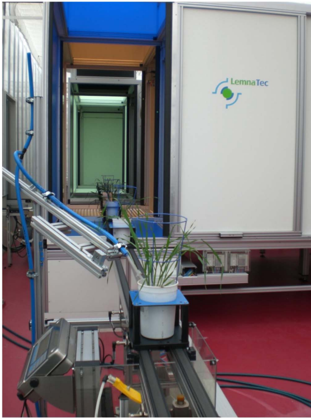
Figure 2. Barley plants at the weighing and watering unit after leaving the imaging station.
