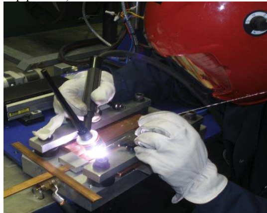
Fig. 3. Photograph of welding engineer carrying out the manual weld build up process.
