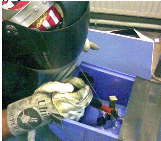
Fig. 5. Photograph of a skilled welding engineer performing a manual weld deposition operation on a compressor blade
