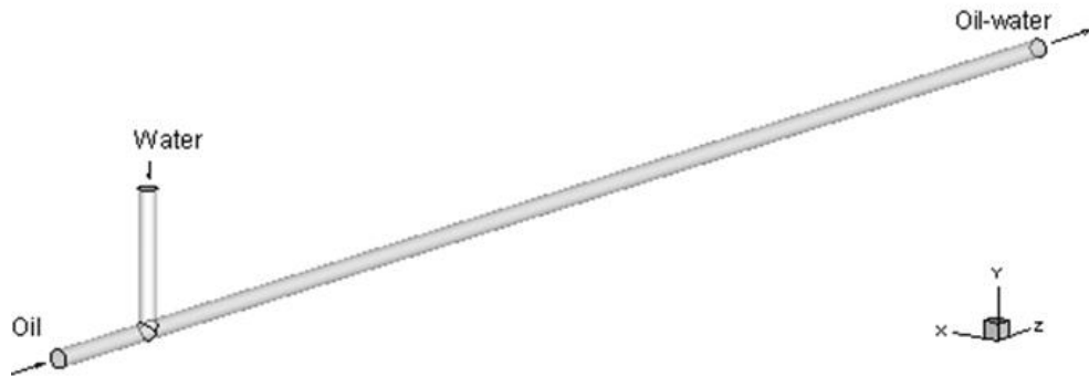
Fig. 2: Pipe geometry for the oil-water flow simulation
