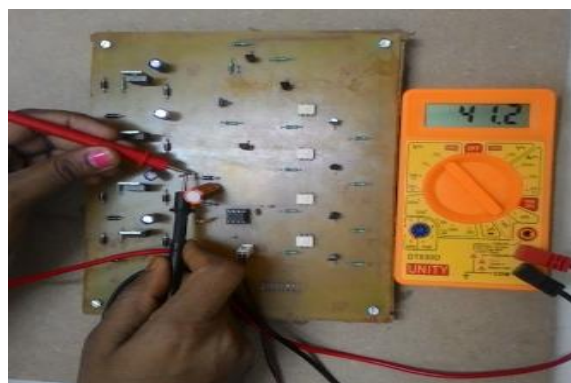
Fig.6 Output of high voltage Marx generator
