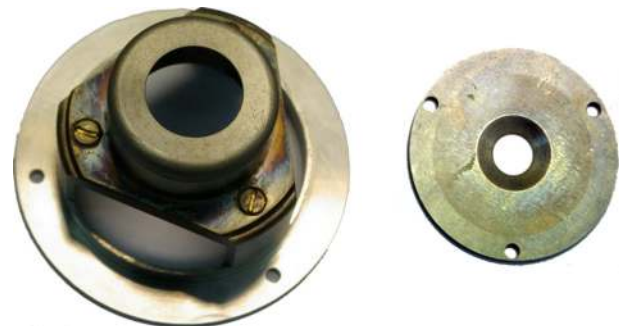
FIG. 2. Puller (on the left), aperture diameter 24 mm; plasma electrode (on the right), aperture diameter 10 mm.
