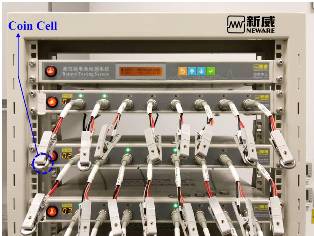
Figure 2 A photograph of the electrochemical lithium ion-intercalation experimental setup (battery test system).
