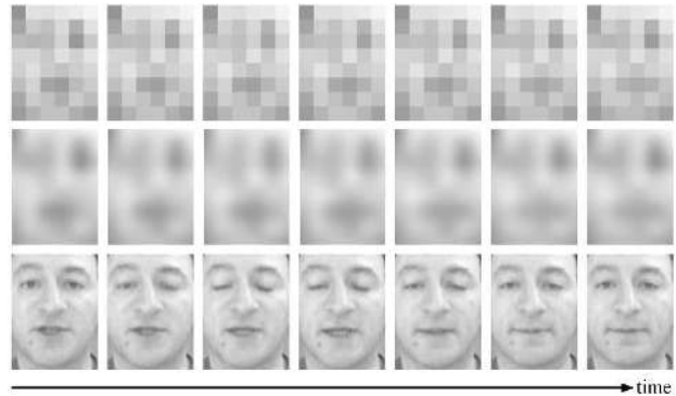
Figure 1: Given only a low-resolution video (top), how can one estimate (or “hallucinate”) the original high-resolution video (bottom)? Unfortunately, simple methods such as bicubic interpolation are insufficient (middle). In this paper we explore zooming using a database of videos with an inference procedure that enforces spatio-temporal consistency of the resulting hallucinated video.
