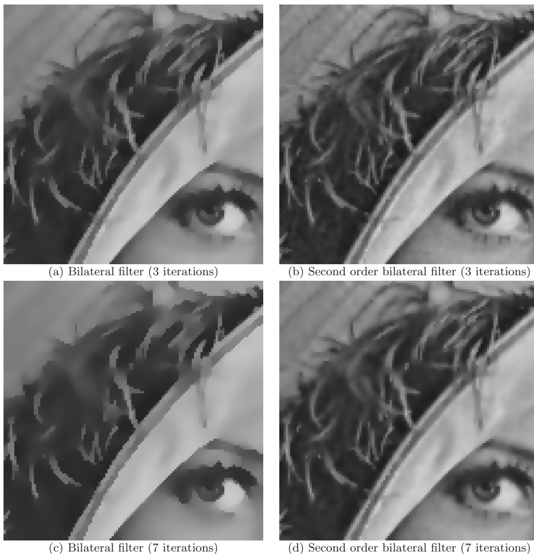
Figure 7. Behavior of iterative higher order bilateral filters: (a) and (c) are the images by applying bilateral filter 3 times and 7 times, respectively, and (b) and (d) are the images by applying second order bilateral filter 3 times and 7 times, respectively. The noise level \text{SNR} = 20[\text{dB}] was used.
