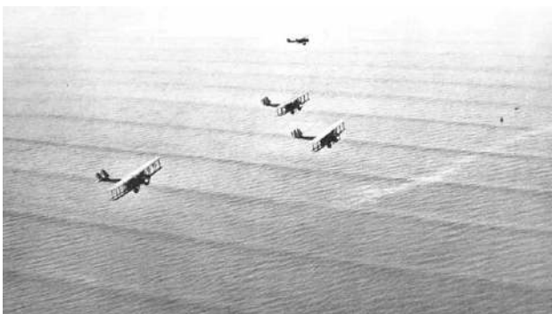
Fig. 1 Cnoidal waves captured by the U.S. Army bombers over the Panama coast in 1933
