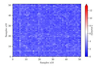
**Figure 6:** Bivariate second-order t-test for the three-share version with 100 000 traces. The t-statistic shows the absolute value.
