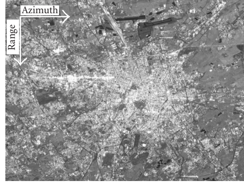
FIGURE 8: Incoherent average of the SAR data available over Milano. Eighty-two images acquired by the ESA-ERS sensors have been processed (Frame 2691-Track 208). The area is heavily urbanized.
