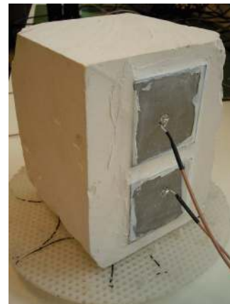
Figure 8 Sample of Newhaven Chalk instrumented with a four-plate capacitive sensor arrangement (two each on the near and far faces) to determine resistivity.
