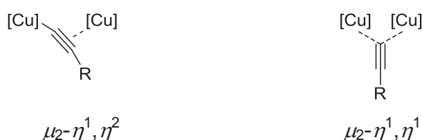
Figure 15: Modes of coordination of a \mu_2 -bridging acetylido ligand in a dinuclear copper complex.
