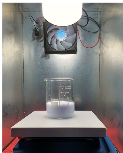
Figure 3. Picture of the photocatalytic reactor used in the experimental procedure.
