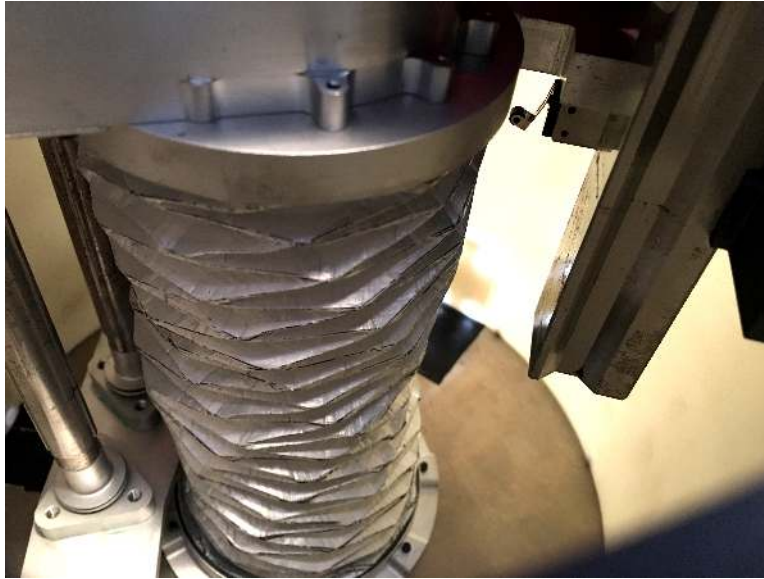
Figure 3.18: Prototype origami-based bellows mounted within Microspine tool.
