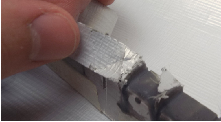
Figure 3.16: Tedlar ® samples tested to failure failed at corners where stress concentrations were greatest.
