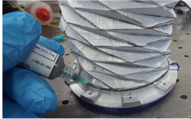
(b) Epoxy being applied to bellows and mount.
