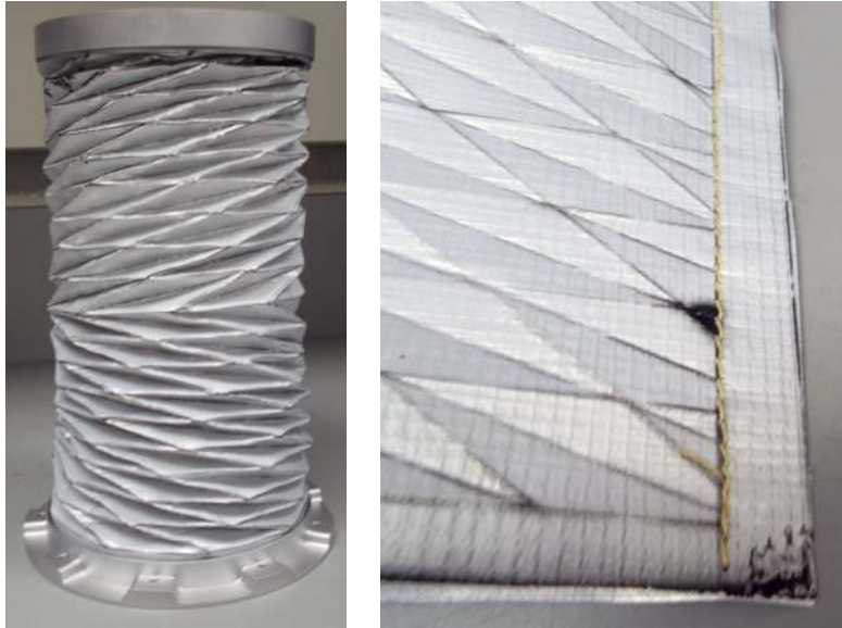
(a) A full sized bellows epoxied within aluminum mounting plates.
