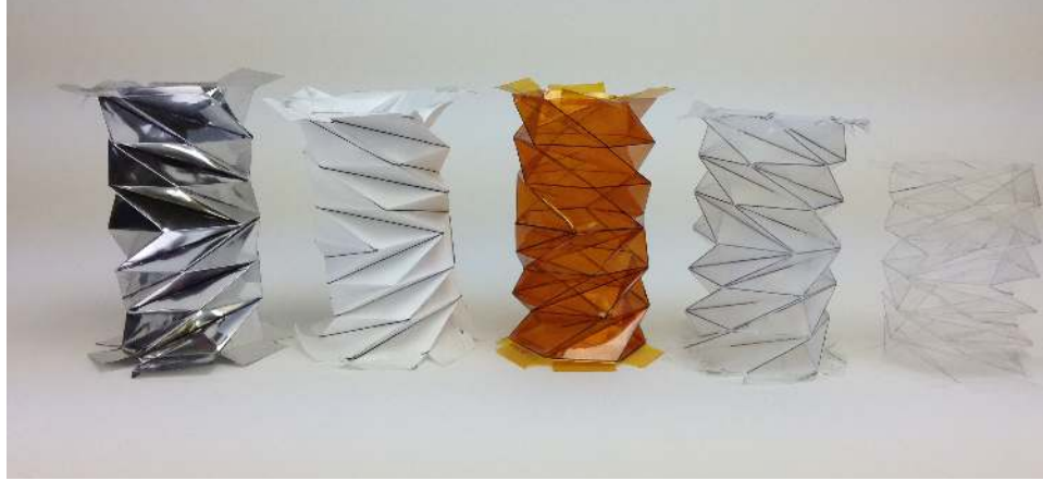
Figure 2.9: Materials tested in the Kresling fold pattern from left to right: Mylar ® , Tyvek ® , Kapton ® , UHMWPE, and ETFE.
