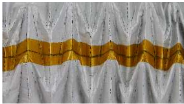
(a) Seam edges placed adjacently and taped.
