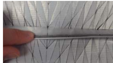
(c) Seam edges overlapped and flanged outward.
