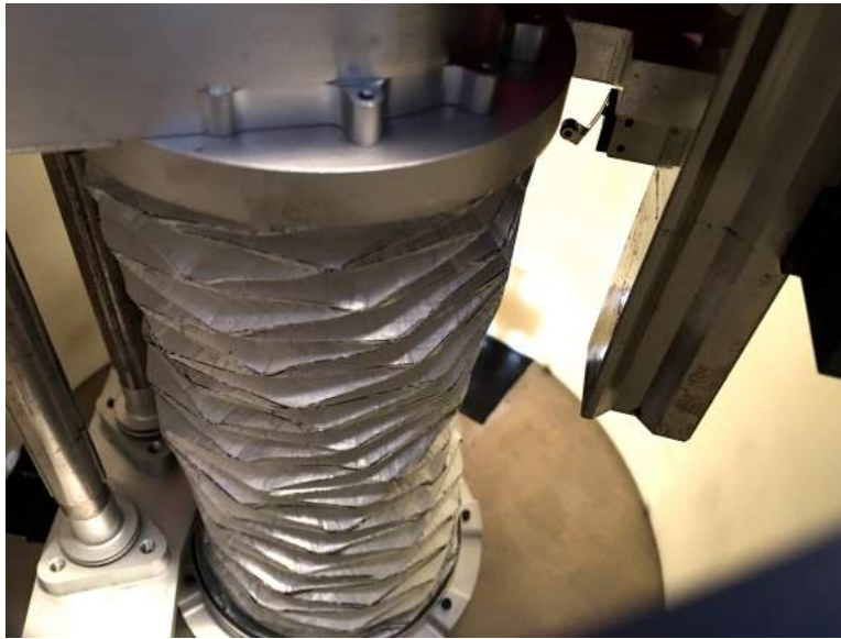
Figure 18. Prototype origami-based bellows mounted within Microspine tool.
