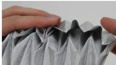
(b) Seam edges overlapped then sealed.
