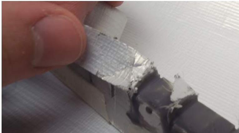
Figure 16. Tedlar® samples failed at corners where stress concentrations were greatest.
