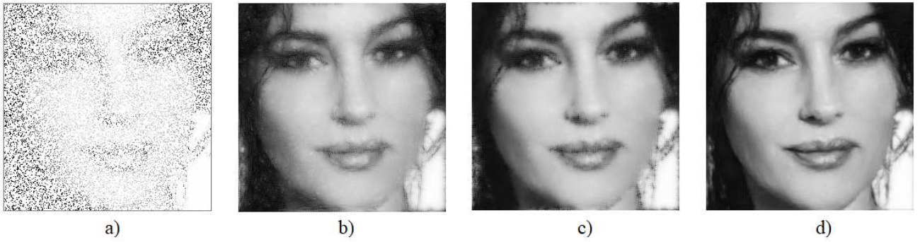
Fig. 9 A comparison of reconstructions of an image with 80% of pixels missing. a) the original corrupted image. b) Reconstruction with the DR method and the hypoelliptic diffusion presented in Section 2. See also [7]. c) Reconstruction with the DR procedure and the varying coefficient hypoelliptic diffusion presented in Section 3. d) reconstruction with the AHE algorithm.
