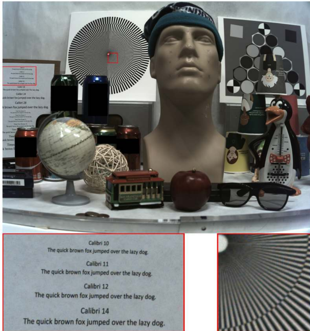
Fig. 9. Image captured with the curved sensor prototype camera. The zoomed-in portion shows excellent sharpness far from center. The large depth range in the scene illustrates pleasing shallow depth of field enabled by the wide aperture of the f/1.2 lens.
