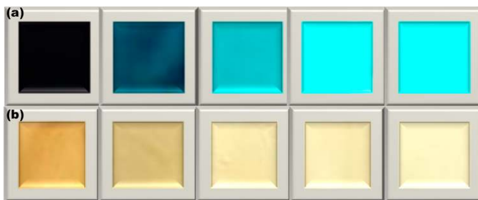
Figure 3. Visual colorimetric detection of TNT. Photograph of the fluorescence quenching of FNFM treated with different concentrations of TNT in aqueous phase when viewed under UV ( \lambda_{\text{ext}}=254 nm) (a) and daylight (b). The tested TNT concentrations are 5 \times 10^{-3} , 5 \times 10^{-4} , 5 \times 10^{-5} , 5 \times 10^{-6} , and 5 \times 10^{-7} M from left to right. The color of the membrane changes from bright bluish-green to blue with increasing concentration.
