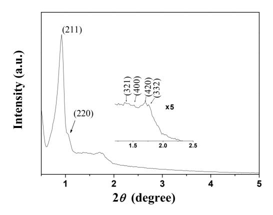
Fig. S1 Small angle X-ray diffraction pattern of KIT-6 template.
