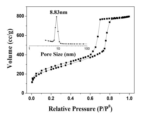
Fig. S2 Nitrogen adsorption/desorption isotherms of KIT-6 template (inset: pore size distribution).
