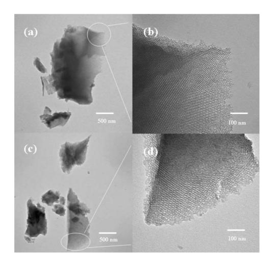
Fig. S3 TEM images of KIT-6 template (a) and (c): low magnification; (b) and (d): high magnification images of selected areas along different directions.
