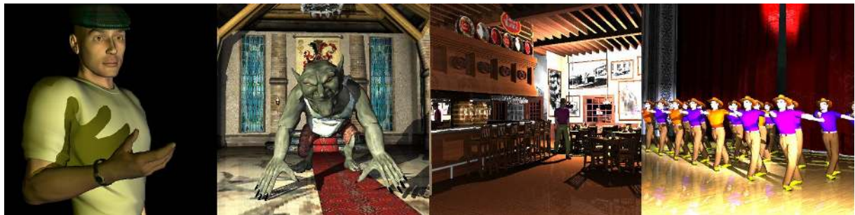
Figure 1: Dynamic scenes ray traced using parallel fast construction of kd-tree. The scenes were rendered with shadows, 1 reflection (except HAND) and textures at 512x512 resolution on a 2-way Intel ®Core™2 Duo machine.
