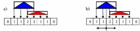
Figure 2: a) Conventional binning algorithms and b) evaluation of SAH using this algorithm
