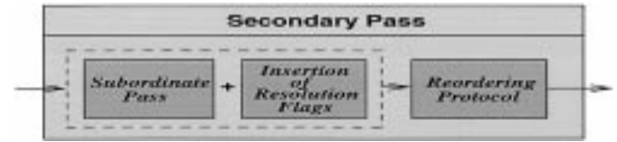
Fig. 9. Secondary pass is made up of three key steps: a subordinate pass, insertion of resolution flags, and a reordering protocol.
