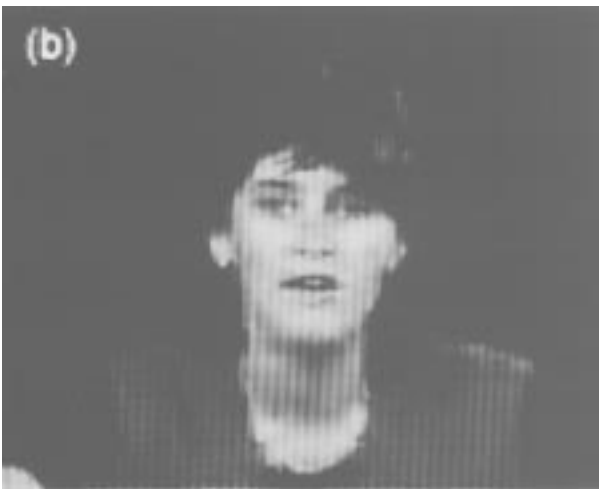
Fig. 14. Miss America frame 64 encoded at 10 Kbits/s by (a) H.263 and (b) TRI-ZTR + MOTION.
