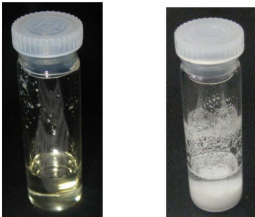
Figure 2. Solubility Comparison of Organocatalysts in \text{CH}_2\text{Cl}_2 . a a The left image illustrates that 300 mg of sulfonamide 1 is soluble in 1 mL of \text{CH}_2\text{Cl}_2 and right image demonstrates that 300 mg of proline is not readily soluble in 1 mL of \text{CH}_2\text{Cl}_2 .
