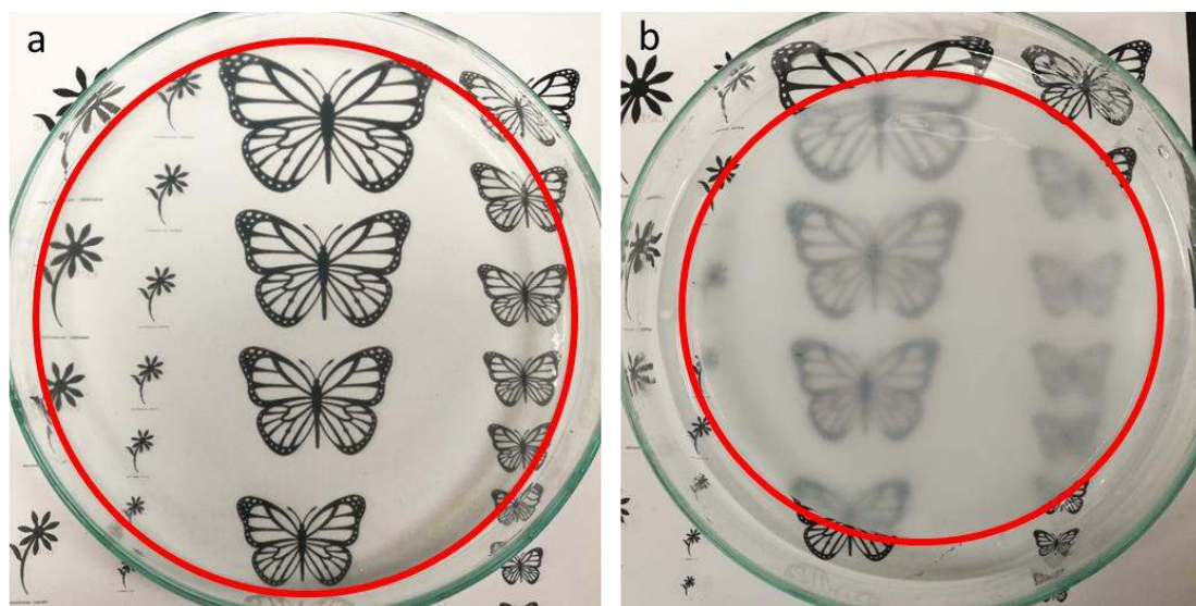
Figure S4. a) PVA-HPC 16% hydrogel, b) PVA-HPC ionic conductive hydrogel (soaked in 5M NaCl solution). After soaking in saturated NaCl solution for 24 hours, volume of PVA-HPC 16% hydrogel decreased from 364 mm 3 to 214 mm 3 . PVA-HPC 16% hydrogel is totally transparent, while PVA-HPC ionic conductive hydrogel is translucent.
