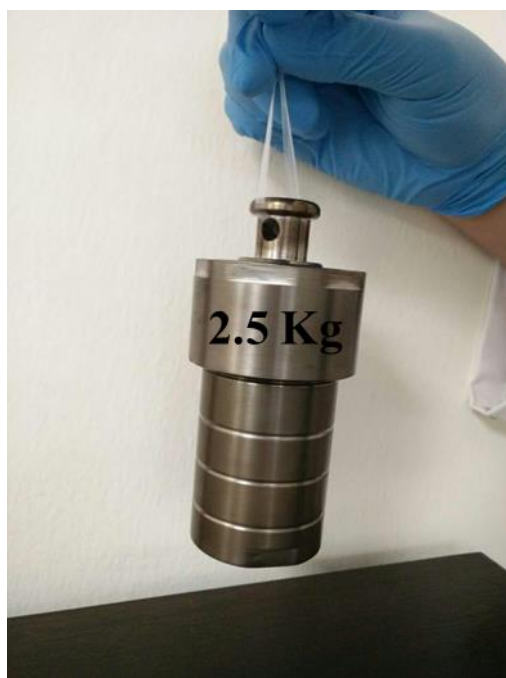
Figure S7. Load-bearing capacity of HPC/PVA ionic conductive hydrogel (3M) (2 mm thickness, 5 mm width).
