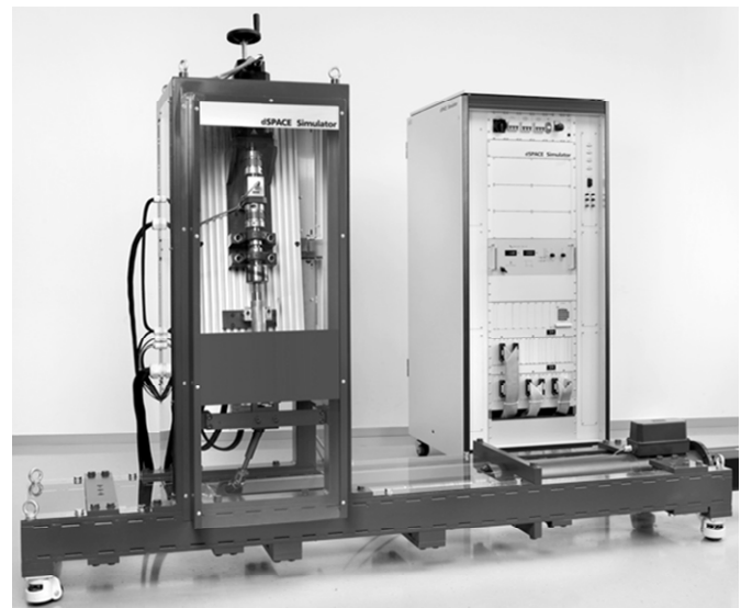
Fig. 3. Mechanical test bench for an EPS including a linear actuator for the steering rod force.
