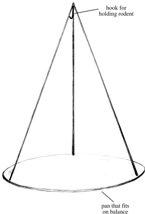
Fig. 5. A tripod used for weighing hindlimb unloaded rats. We use a string of paper clips attached to the hook to adjust for height. The forelimbs of the rat should touch the balance.
