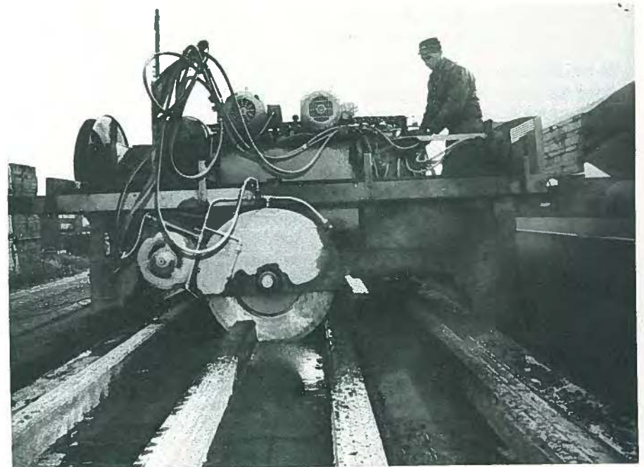
Fig. 26. After the concrete set, the Quadeck was cut to size by a saw attached to the machine.
