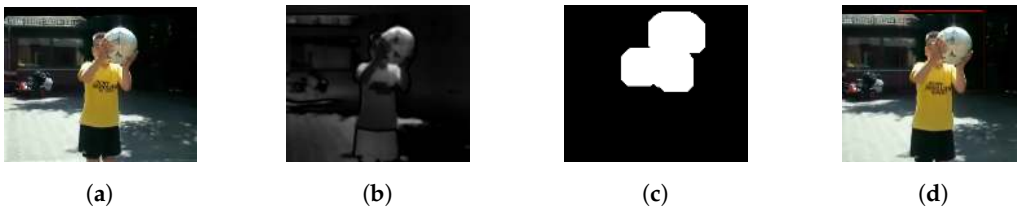
Figure 3. Moving Object Detection: (a) Video Sequence. (b) Saliency Map. (c) Silhouette Creation. (d) Segmented Object Image.
