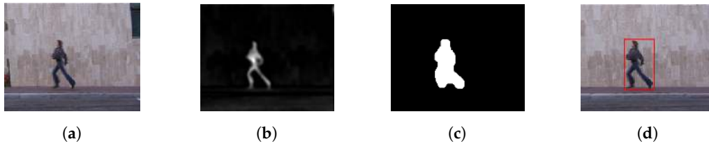
Figure 2. Moving Object Detection: (a) Video Sequence. (b) Saliency Map. (c) Silhouette Creation. (d) Segmented Object Image.
