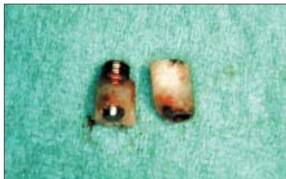
Fig 3 (Right) Retrieved implants demonstrating bone resorption, which is especially notable on (left) the turned implant modification.
