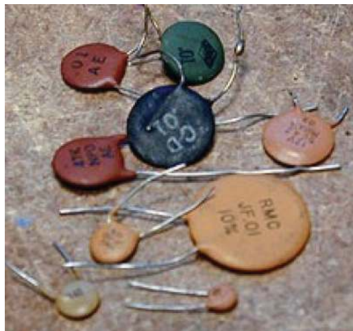
Figure 4. Examples of early ceramic capacitors taken from antique radios. Early ceramic capacitors looked very much like modern examples, although somewhat larger for a given capacitance. Then, as now, ceramic capacitors were very reliable. Photo courtesy of P. I. Nelson, www.antiqueradio.org , and used with permission.
