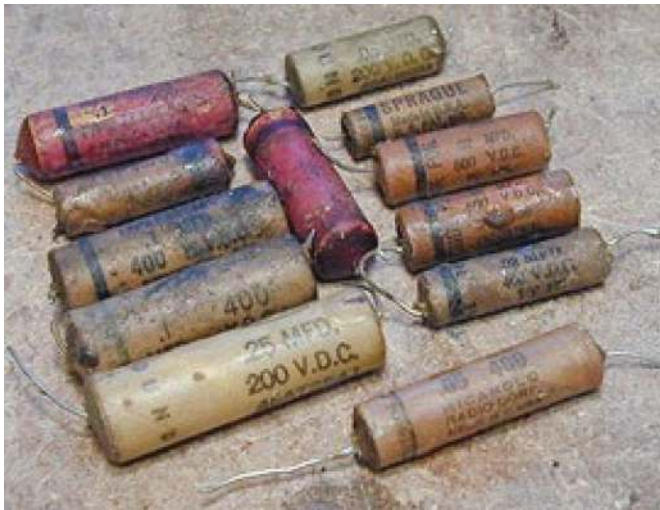
Figure 1. Examples of early waxed paper and foil capacitors taken from antique radios. Such capacitors tend to be unreliable and are usually replaced with metalized polymer film capacitors when restoring a radio. Photo courtesy of P. I. Nelson, www.antiqueradio.org , and used with permission.
