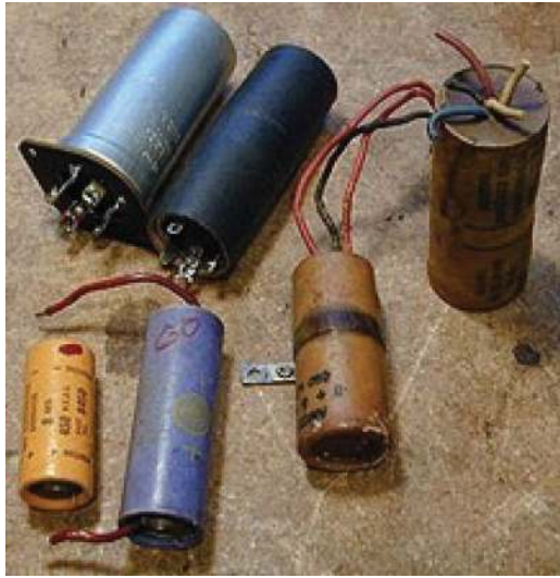
Figure 3. Examples of early electrolytic capacitors taken from antique radios. These capacitors are also unreliable and are replaced when restoring such a radio. Photo courtesy of P. I. Nelson, www.antiqueradio.org , and used with permission.
