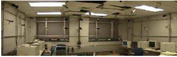
Figure 3: 3D Room : the Virtualized Reality setup with digital capture [14].
