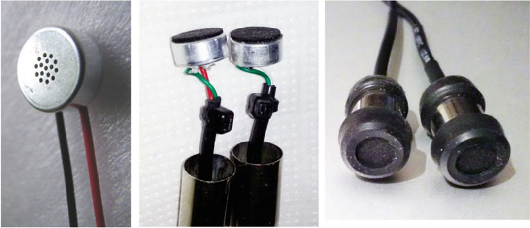
Fig. 1.13 Photograph of the PRIMO EM172 microphone capsule (left) used by many nature sound recordists for their custom-made microphones (center and right). Courtesy of M Pesente
