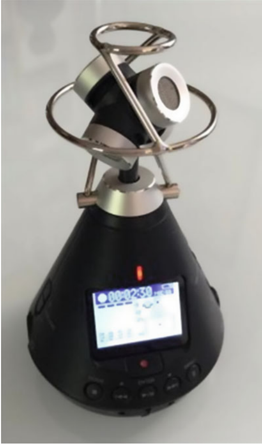
Fig. 1.14 Ambisonic recorder with 4 microphones (first order) Zoom H3VR
