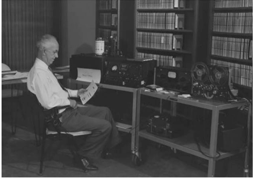
Fig. 1.22 Photograph of L. Irby Davis using an early Kay Electric Co. Sona-Graph Sound Spectrograph analyzer (the late 1950s). Notice the sonogram on the paper wrapped around the drum on top of the analyzer. Courtesy of the Cornell Laboratory of Ornithology
