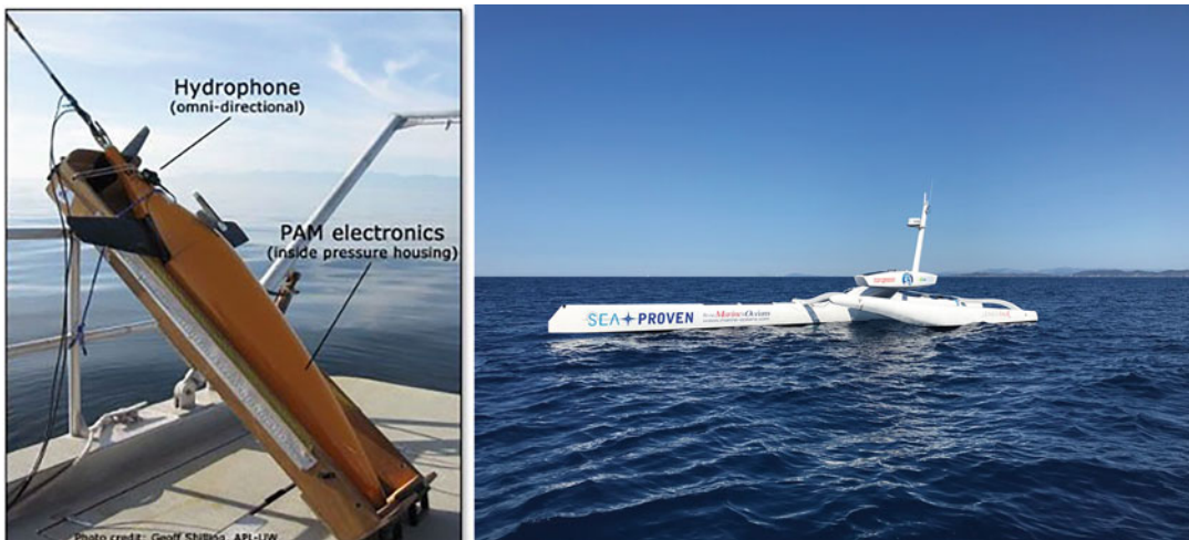
Fig. 1.20 Left: Photograph of the passive acoustic seaglider™ developed by the Applied Physics Laboratory, University of Washington. Courtesy of G Shilling. Right:
