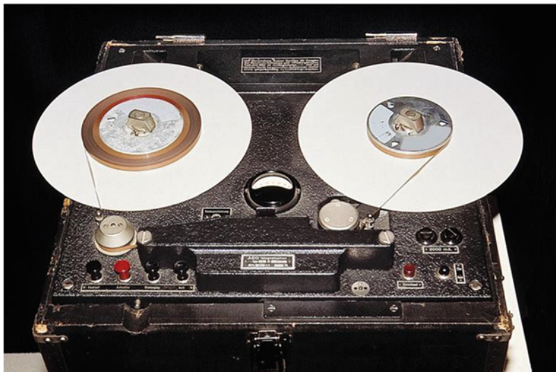
Fig. 1.5 Open-reel recorder made by AEG (1939). Image source: https://commons.wikimedia.org/wiki/File:AEG_Magnetophon_K4_1939.jpg , by Friedrich Engel, CC
