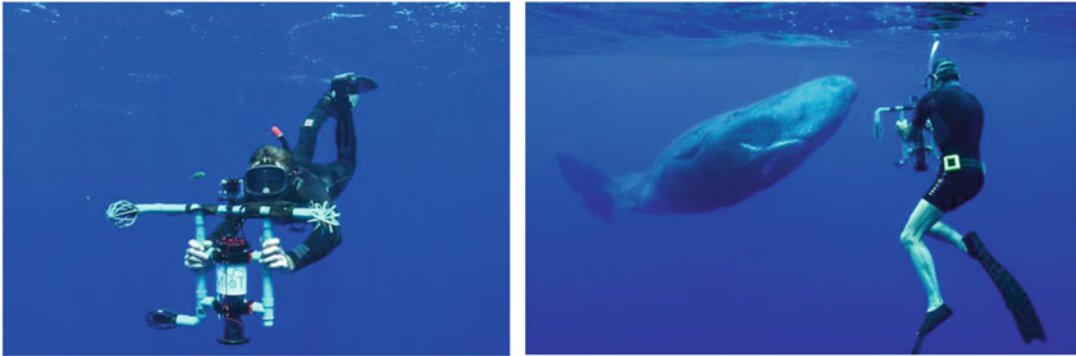
Fig. 1.19 The JASON Qualilife DAQ 3x600 kHz in the custom array by H Glotin, recording sperm whales in the near field in 2018. Courtesy of V Sarano
