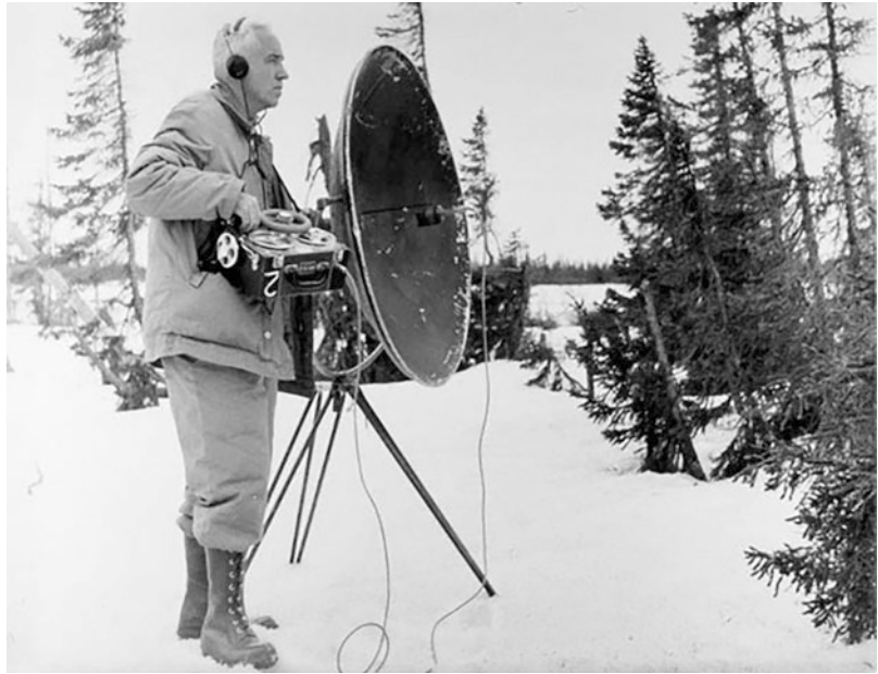
Fig. 1.6 Photograph of an early 1950s field recording system. Peter Paul Kellogg with an Amplifier Corporation of America Magnemite 610 reel-to-reel tape recorder and a Western Electric 633 microphone mounted in a parabolic reflector. Courtesy of the Cornell Laboratory of Ornithology
