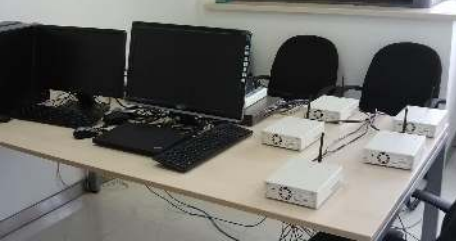
Fig. 5. Overview of the evaluation environment. 5 USRP2 devices are used in our experiments and the evaluation is conducted in an indoor environment.
