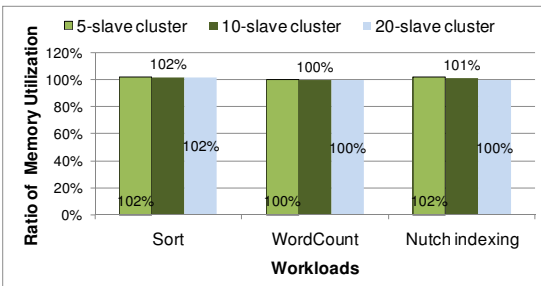
Figure 12. Ratio of instrumented cluster memory utilization over baseline cluster memory utilization
