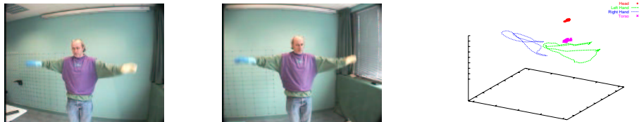
Figure 2: Left: Example of images of the “Vinci” sequence from the point of view of the left camera (on the left) and from the point of view of the right camera (on the right). Right: 3D coordinates of the center of each blob (head, torso, left hand and right hand) for a “swim” gesture.
