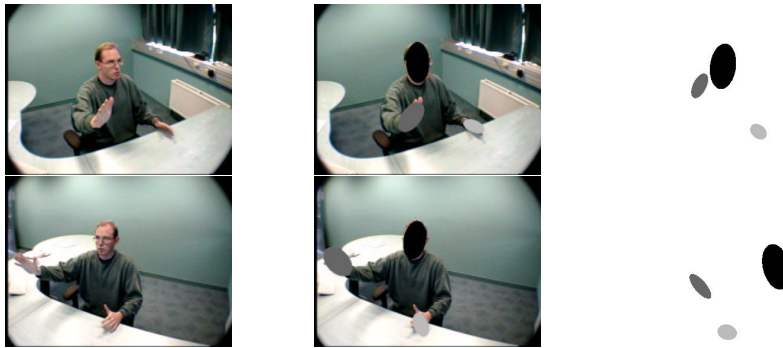
Figure 1: Left: left and right captured images. Center: left and right images with projected ellipsoids. Top right: ellipsoids projection on the frontal plane. Down right: ellipsoids projection on the side plane (the cameras are on the left side).
