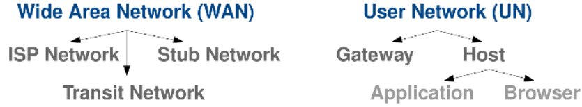
Fig. 1. A taxonomy for broadband performance evaluation approaches based on the location of the VPs initiating the measurements.
