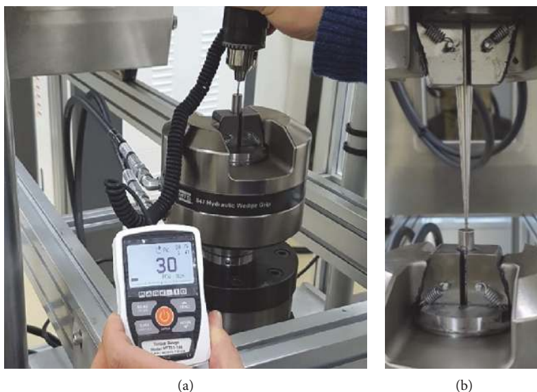
FIGURE 2: Example of mechanical test. (a) Fixed abutment screw on the jig by applying insertion torque. (b) Vertical loading.
