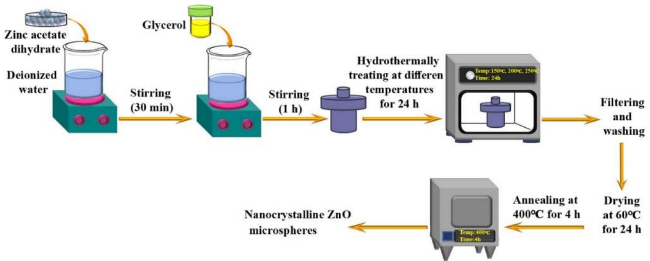
Fig. 1 Schematic representation of the synthetic procedure for the preparation of ZnO microspheres
