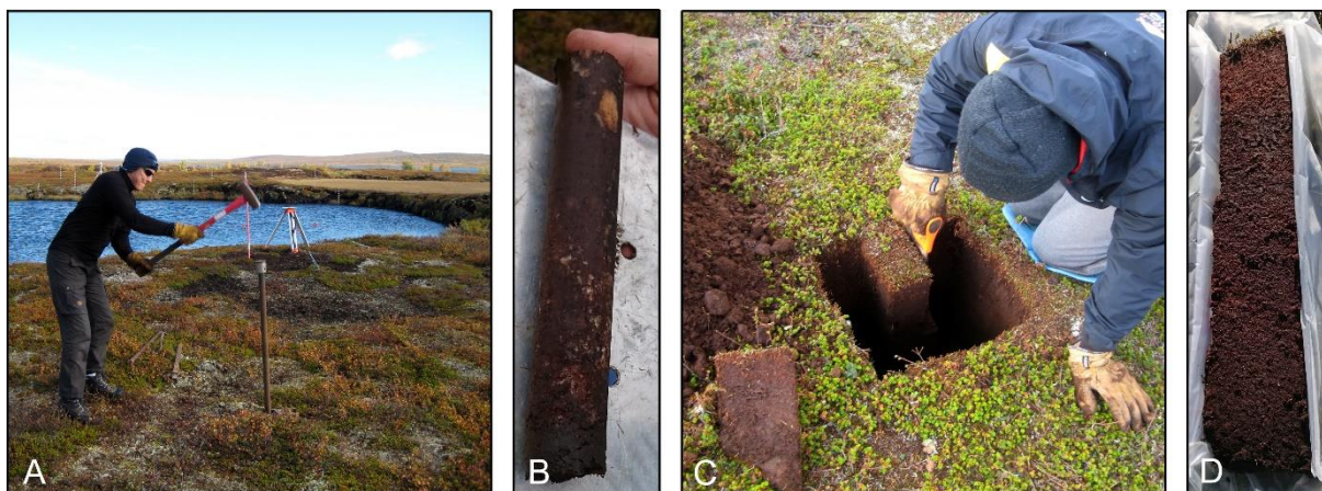
Fig. 2. Field sampling methods. Sampling with steel pipes (A), and collected material (B). Sampling using a saw (C) to cut out blocks of peat (D).
