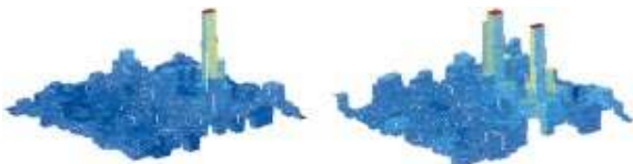
Fig. 9. MOT-induced fluorescence of single atoms confined in distinct dipole traps of a three-trap array, where the traps are separated by a few micrometers. The two figures show one atom captured in one of the traps and two atoms being simultaneously trapped in two traps of a three-trap array. The integration time of the CCD was set to 200 ms.
