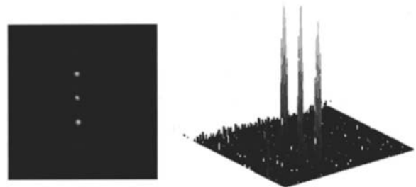
Fig. 5. Two-dimensional and three-dimensional plots of the intensity profile generated by a three-spot hologram. The image was captured by focusing the diffracted beams onto a CCD camera by use of an auxiliary lens with 160-mm focal length.
