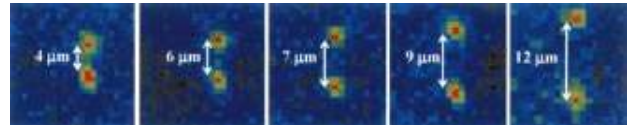
Fig. 8. MOT-induced fluorescence of trapped atoms in two dipole traps. The integration time of the CCD is 200 ms. The figures show how the distance could be varied with micrometer accuracy by sending a modified signal to the SLM.
