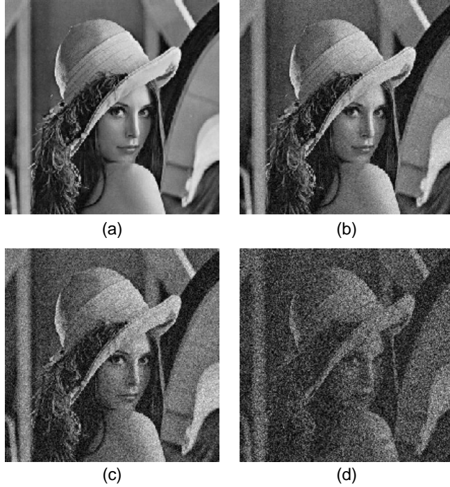
Figure 2. The decrypted 2D image with (a) no quantization, and decrypted with (b) 64, (c) 8, and (d) 2 quantization levels in the phase mask.
