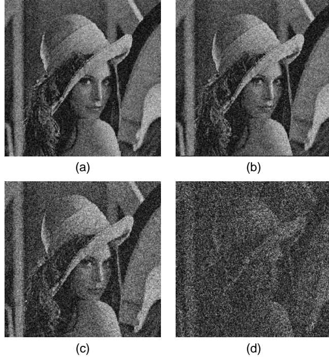
Figure 3. The decrypted 2D image after the phase-only encrypted image is quantized to (a) 128, (b) 8, (c) 4, and (d) 2 phase levels.
